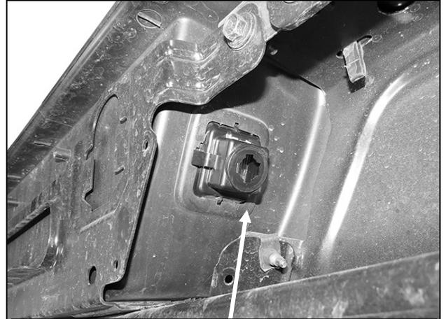
**(Fig 2) Unplug and remove license plate lights**
