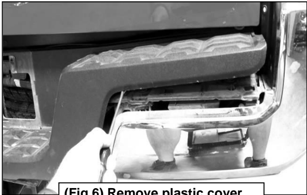
(Fig 6) Remove plastic cover from the top of the bumper
