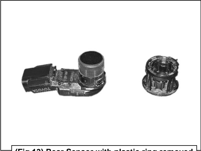
(Fig 13) Rear Sensor with plastic ring removed
