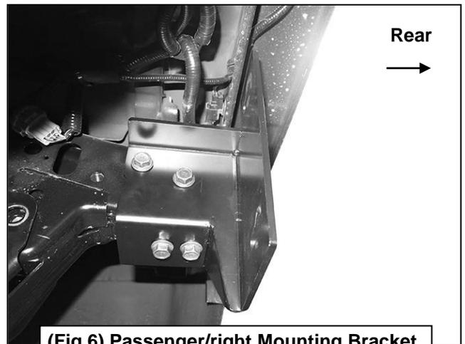
**(Fig 6) Passenger/right Mounting Bracket installed on model without hitch**
