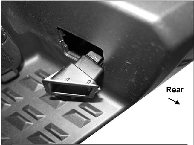
**(Fig 16) Unplug license plate lights and trailer connector. Remove lights and**
