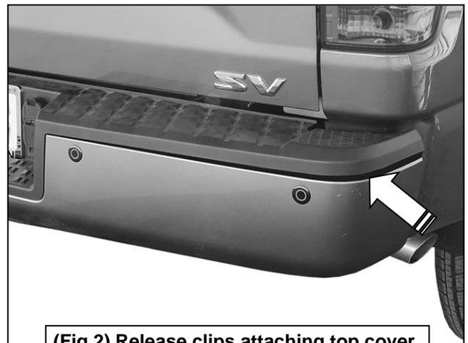
**(Fig 2) Release clips attaching top cover**
