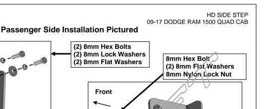
(Fig 12) Attach passenger/right front Support Bracket to front facing side of Mounting Bracket
