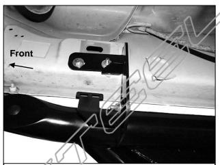
(Fig 11) Passenger side front on models with factory installed threaded inserts. Bolt Plate not required
