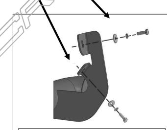
(Fig 6) Driver Side Front Bracket Installation of parts for Vehicle years 2016 and above
