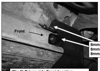
8mm x 30mm Hex Bolt 8mm Lock Washer 8mm x 24mm Flat Washer
