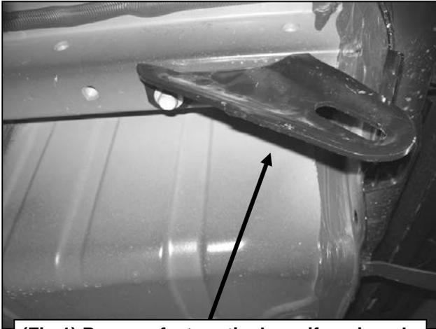
**(Fig 1) Remove factory tie down if equipped**
