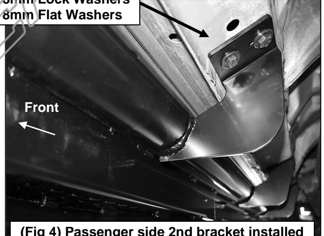
(Fig 4) Passenger side 2nd bracket installed
