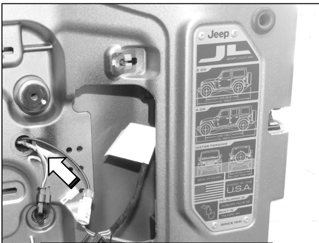
(Fig 3) Disconnect the wires and pull the wires out through the hole
