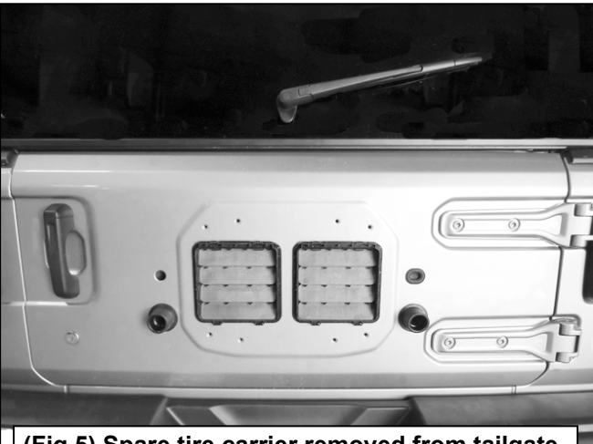
(Fig 5) Spare tire carrier removed from tailgate
