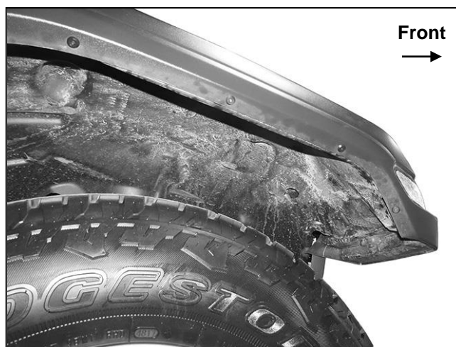
(Fig 2) Remove hardware attaching fender liner to front, top and back of fender (passenger/right side pictured)
