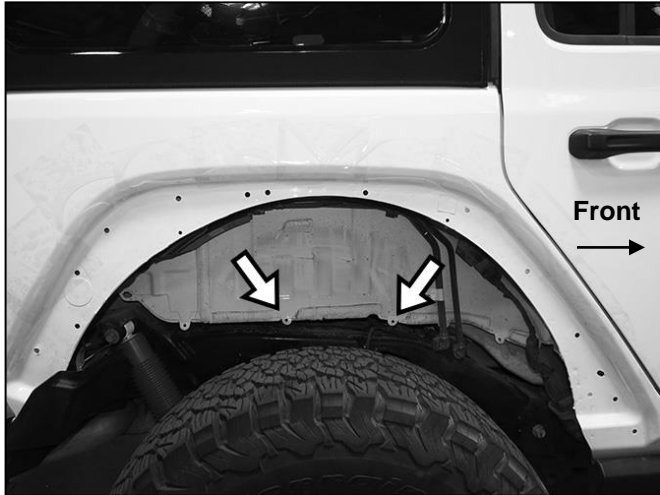
(Fig 4) Attach Fender Liner to the (2) 6mm Clip Nuts with the included (2) 6mm Combo Bolts (arrows)
