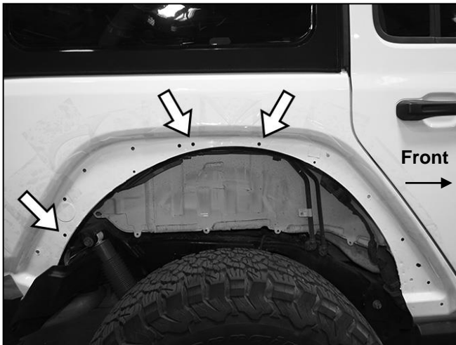
(Fig 3) Fender Liner will attach to the (3) factory locations typically used to attach aftermarket fenders (arrows). Attach the Fender Liner to these mounting points, (passenger/right side pictured without fender for instruction purposes only)
