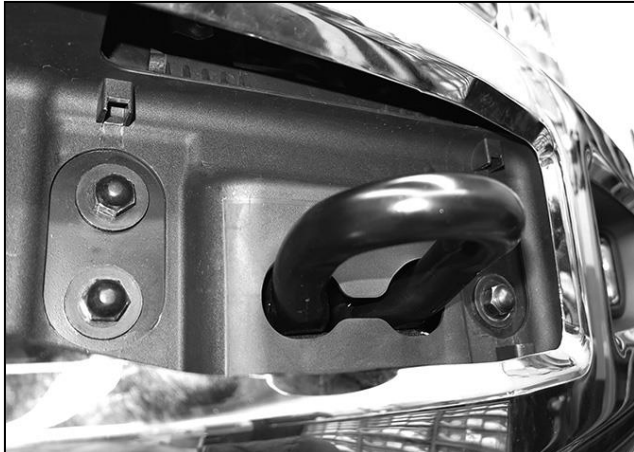
(Fig 6) Remove bumper bolts (driver side pictured)
