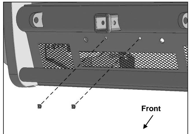
(Fig 18) Attach License Plate Plugs to Bumper
