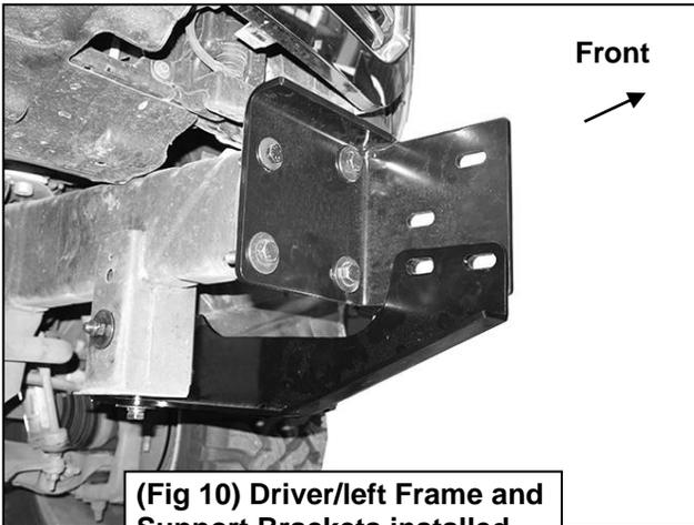
(Fig 10) Driver/left Frame and Support Brackets installed
