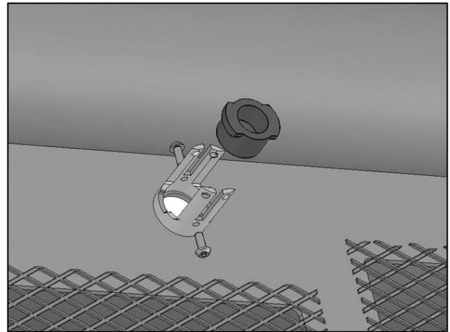
(Fig 11) Push Rubber Plug into mounting sleeve
