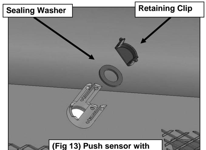
(Fig 13) Push sensor with Sealing Washer into sleeve
