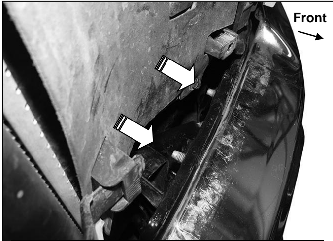
(Fig 3) Remove driver side top bumper hardware
