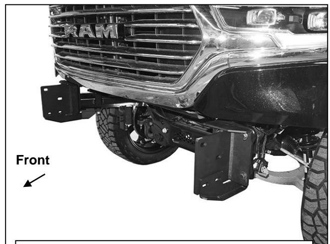
(Fig 8) Frame and Support Brackets installed
