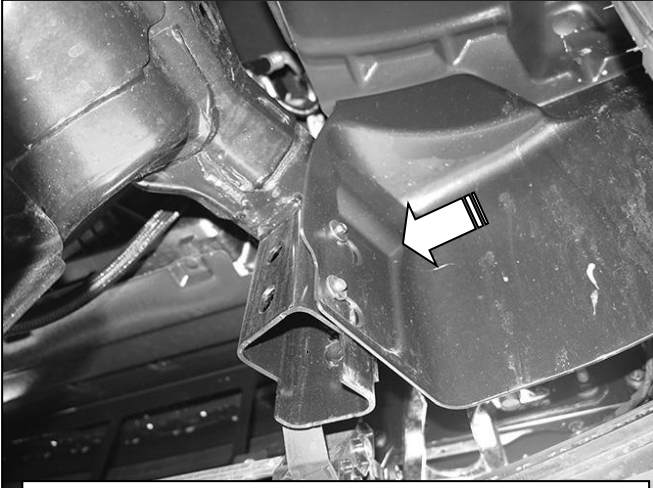
(Fig 1) Remove screws attaching plastic splash guard to frame. Passenger/Right side pictured
