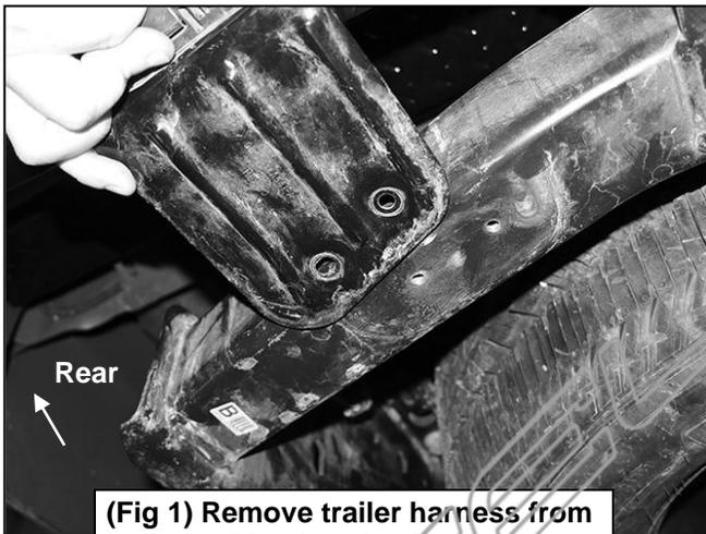
**(Fig 1) Remove trailer harness from bottom of hitch or back of bumper**
