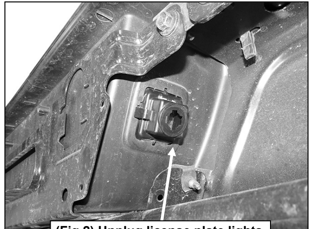
(Fig 2) Unplug license plate lights
