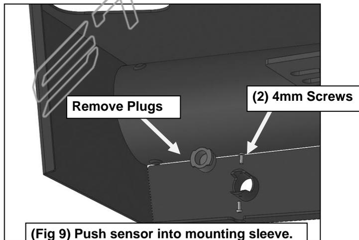
(Fig 9) Push sensor into mounting sleeve. Use 4mm Screws to lock sensor in place.
