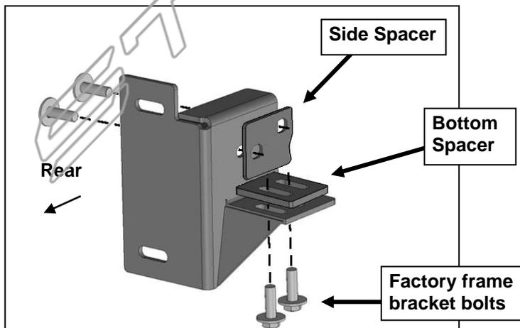
(Fig 5) Passenger/right side Mounting Bracket w-o hitch
