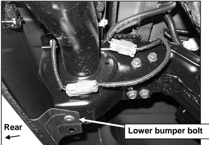
(Fig 1) Unplug wiring harnesses (driver side pictured)
