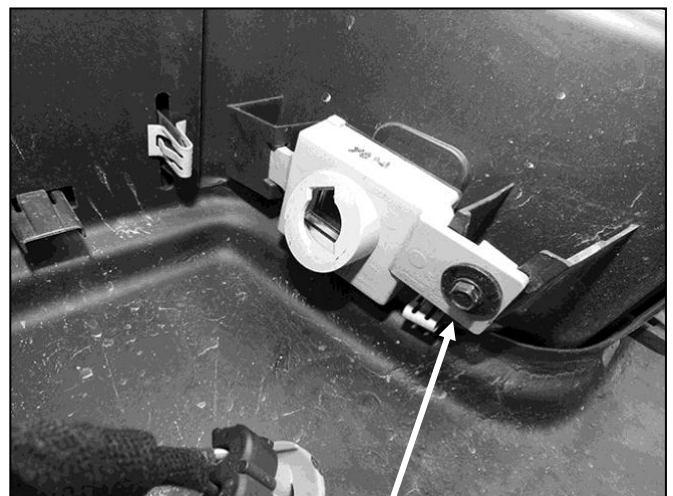
(Fig 4) Remove license plate lights and wiring harness from factory bumper
