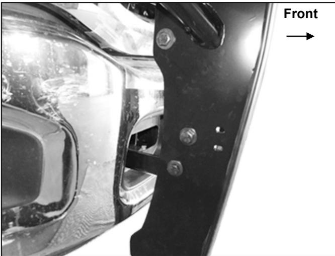
**(Fig 14) Attach Grill Guard to outside of Mounting Brackets (passenger/right side pictured)**
