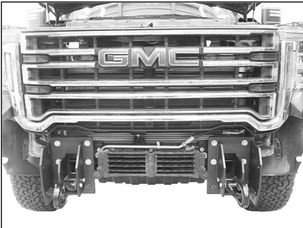
(Fig 20) Tow hooks and all Brackets installed.
