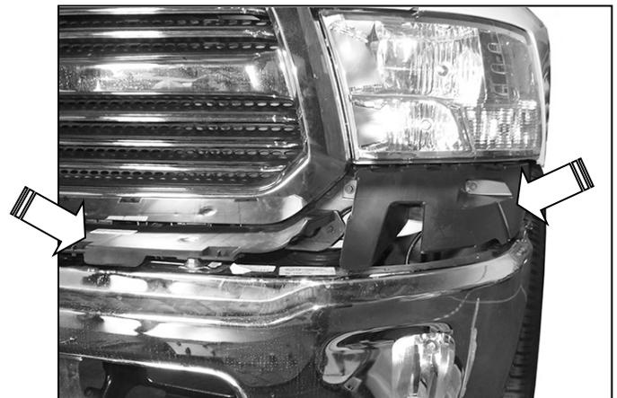
(Fig 3) Remove fascia body panel from top of bumper, (arrows) or 1pc plastic bumper cover
