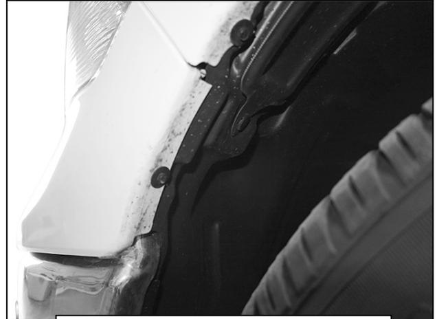
(Fig 2a) Remove hardware attaching plastic fender liner to fender
