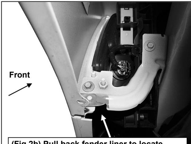
(Fig 2b) Pull back fender liner to locate fascia attachment at bottom of front fender
