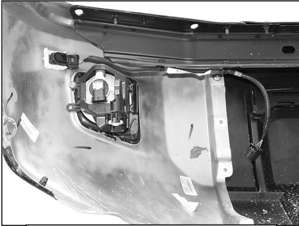
(Fig 16) Remove sensor and fog light
