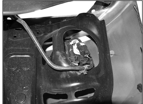
(Fig 7) Disconnect and move wiring harness away from bumper (passenger/right side)
