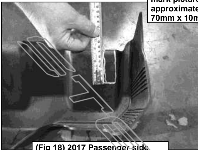
(Fig 18) 2017 Passenger side DEF cover marked for trimming
