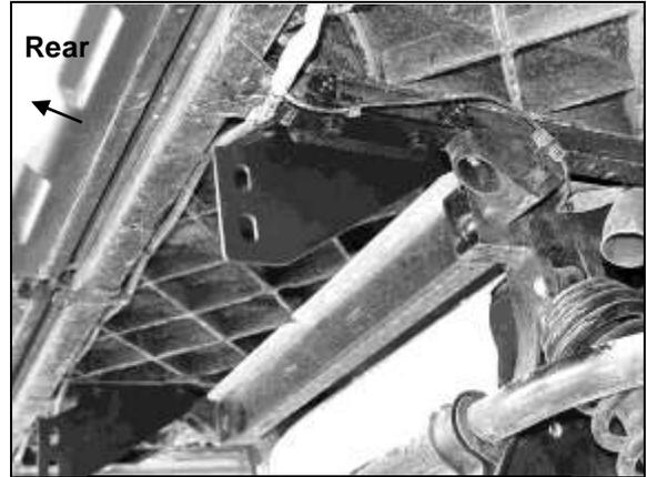
**(Fig 9) Frame Brackets installed**
