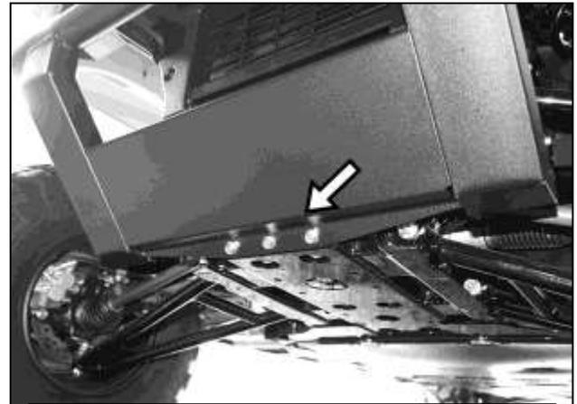
(Fig 2) Remove lower bumper bolts (arrow)
