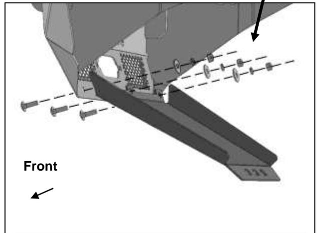
**(Fig 7) Attach Bumper to front of Skid Plate**
