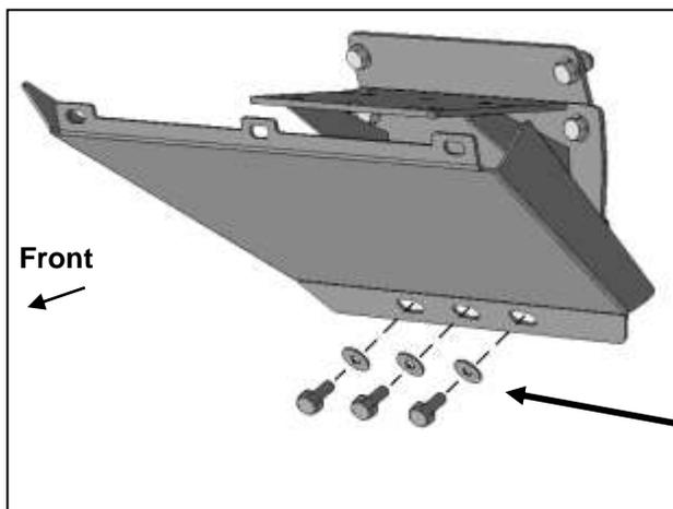
(Fig 5) Attach bottom of Skid Plate to front of frame
