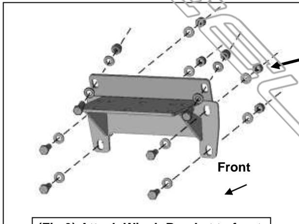
(Fig 3) Attach Winch Bracket to front of frame (installation optional)
