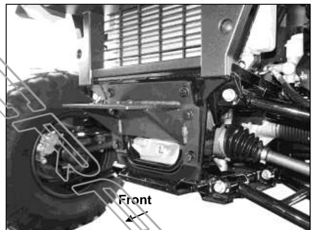
(Fig 4) Winch Mount installed
