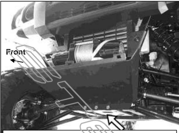
**(Fig 6) Winch Mount and Skid Plate installed**
