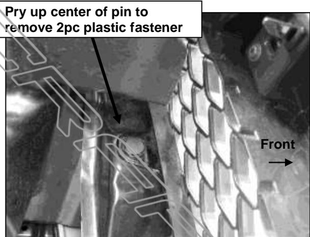
Pry up center of pin to remove 2pc plastic fastener
