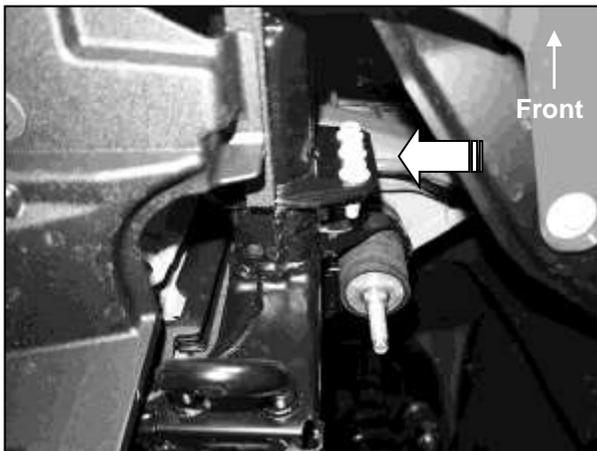
(Fig 3) Remove (3) factory bumper bracket
