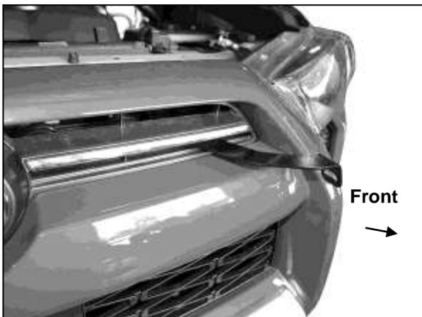
**(Fig 14) 2014-on, driver/left Top Bracket installed**
