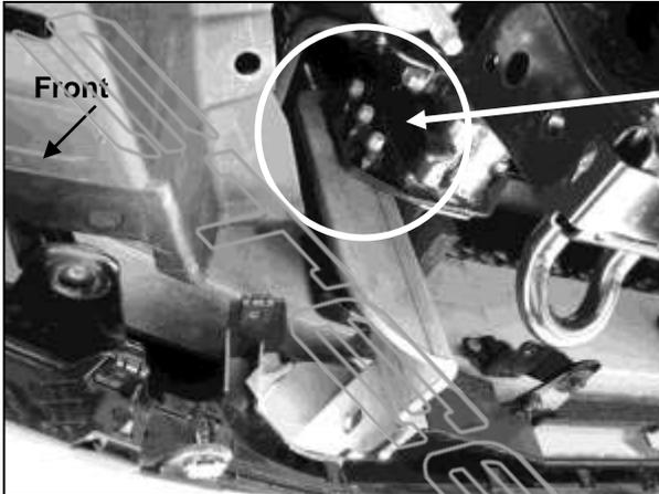
Reuse factory bolts to attach Frame Bracket to bumper bracket
