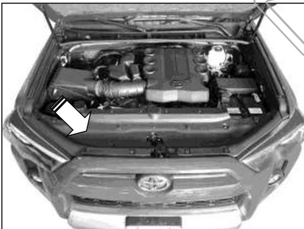
**(Fig 7) Remove plastic cover (arrow)**
