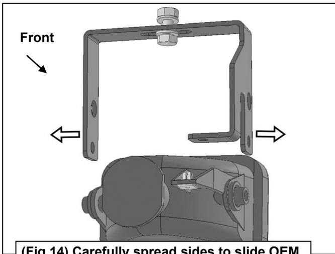
(Fig 14) Carefully spread sides to slide OEM fog light into position in pivot holes
