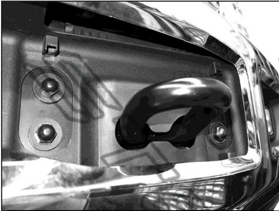
(Fig 6) Remove bumper bolts from front
