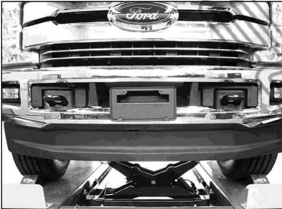
(Fig 3) Remove plastic air dam from bumper
