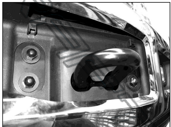
(Fig 4) Remove bumper bolts (driver/left side pictured)
