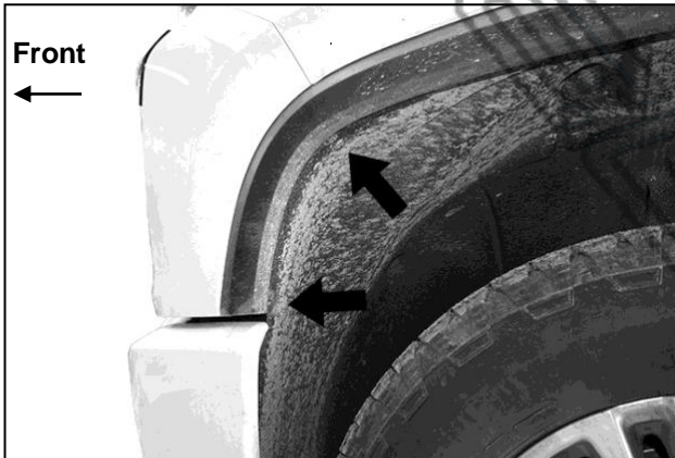
(Fig 1) Release hardware attaching fender liner from plastic panel (fascia-see arrows)
