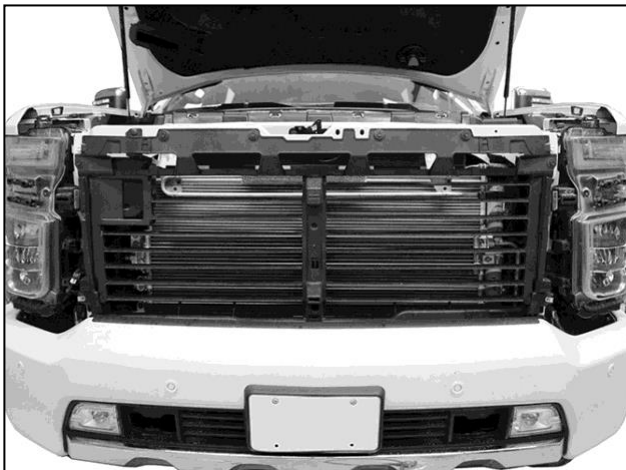
(Fig 7) Grille and fascia removed
