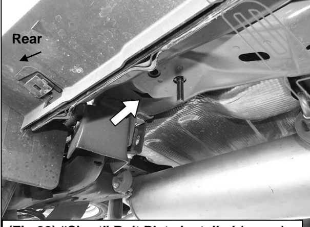
(Fig 22) "Short" Bolt Plate installed (arrow)
