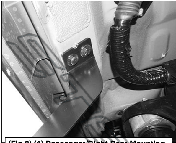
(Fig 8) (1) Passenger/Right Rear Mounting Bracket attached to the rear location
