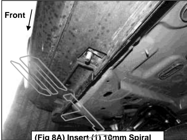
(Fig 8A) Insert (1) 10mm Spiral Bolt into the side panel
