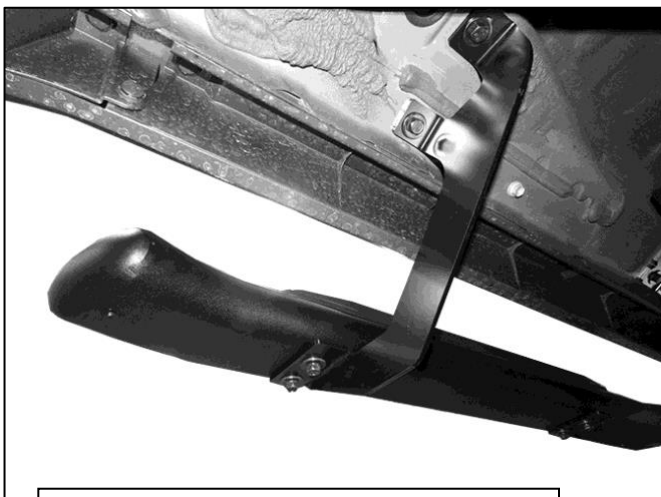
(Fig 10) Passenger/Right Sidebar attached to the Front Mounting Bracket
