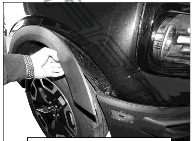
(Fig 6) Gently but firmly, pull the front of the fender out from the bumper
