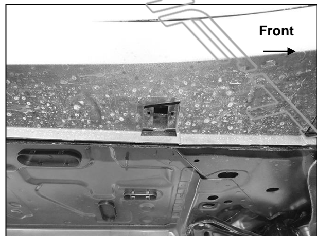
(Fig 2) Passenger/right #2 clip removed
