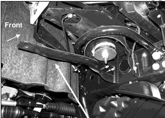
(Fig 5) Remove outer bumper support brackets
