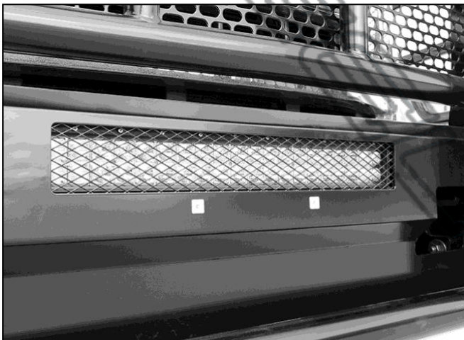
(Fig 19) Push plastic plugs into holes in Bumper for license plate if required. LED bar light pictured installed behind Bumper on non-ecoboost model. LED light installation not recommended on ecoboost models
