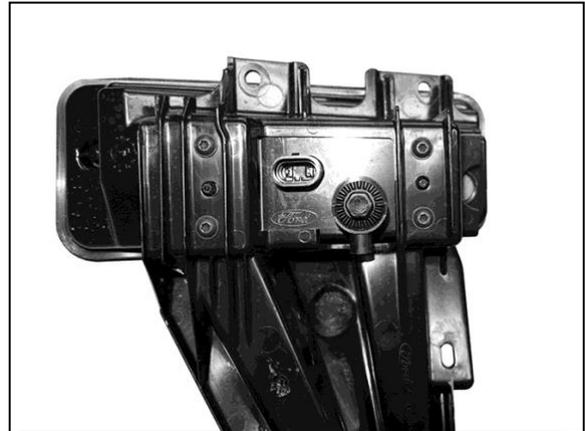
(Fig 19) Remove screws to remove narrow LED fog light from plastic mount
