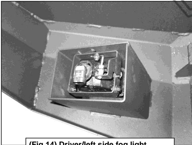
(Fig 14) Driver/left side fog light assembly attached to back of Bumper
