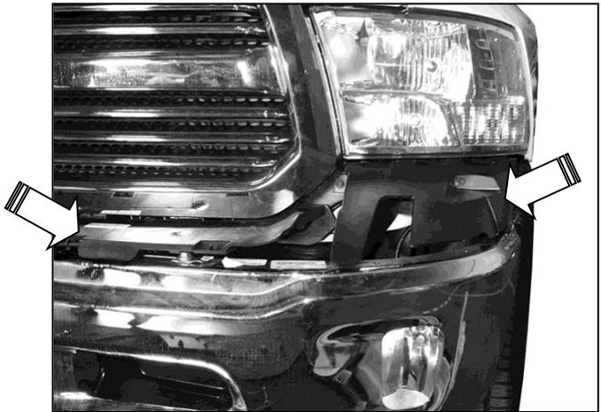
(Fig 4) Remove fascia body panel from top of bumper, (arrows) or 1pc plastic bumper cover
