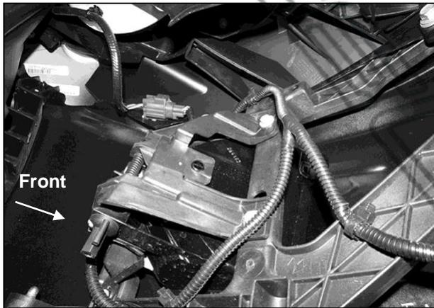
(Fig 5) Unplug lights and sensors if equipped. Unplug harness to bumper and move harness
