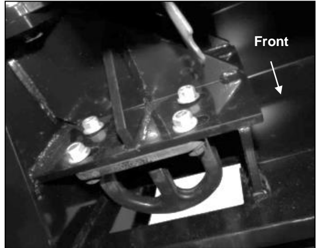
(Fig 14) Reuse factory hardware to attach tow hook to mounting plates on Elevation Bumper. NOTE: Preproduction Bumper pictured from below for instruction purposes, actual Bumper may differ slightly
