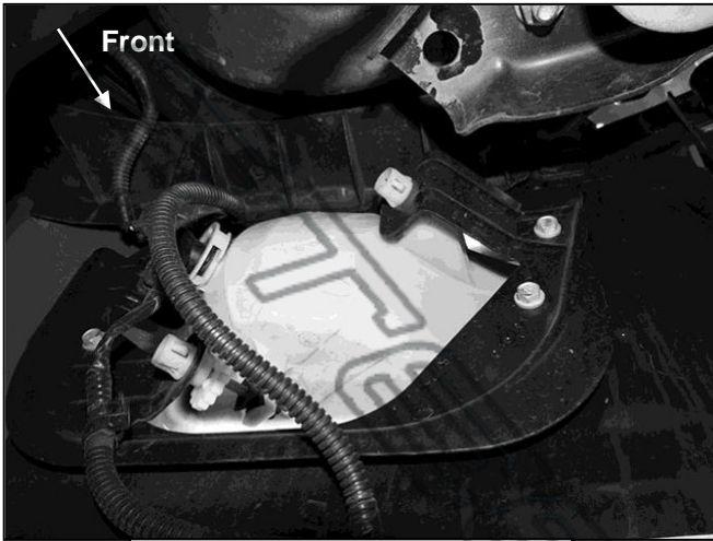
(Fig 1) Unplug wiring harness leading to front bumper
