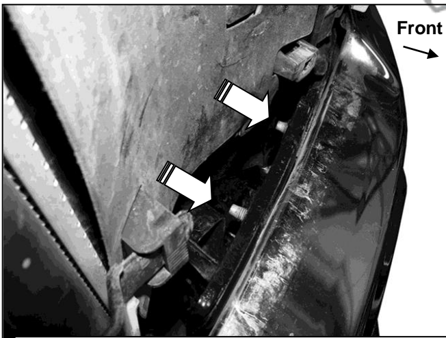
(Fig 3) Remove driver side top bumper hardware
