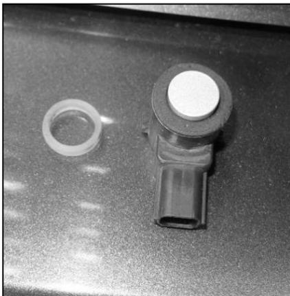
(Fig 10) Replace factory seal washer with Foam Washer
