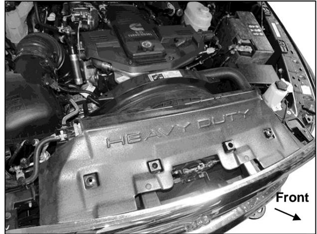
(Fig 2) Open hood and remove plastic cover
