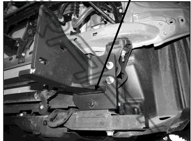
(Fig 9) Driver/left Mounting Bracket attached to end of frame
