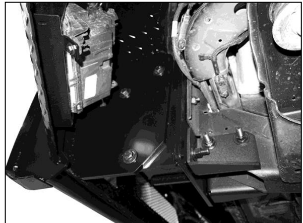
(Fig 24) Driver/left side of Bumper installed
