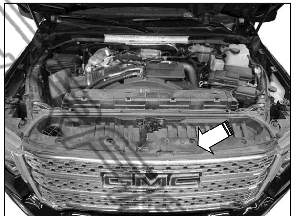
(Fig 2) Remove hood release handle and cover. Reinstall handle. Carefully remove grille. Models equipped with grille mounted camera, pull grille forward and unplug camera
