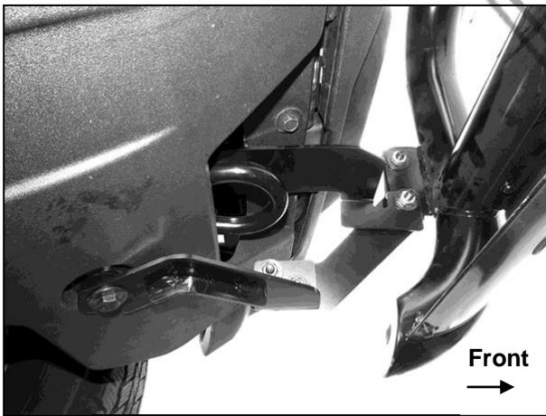
(Fig 13) Driver/left side of Bull Bar attached to Brackets
