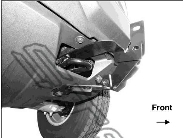
(Fig 11) Driver/left side Brackets installed
