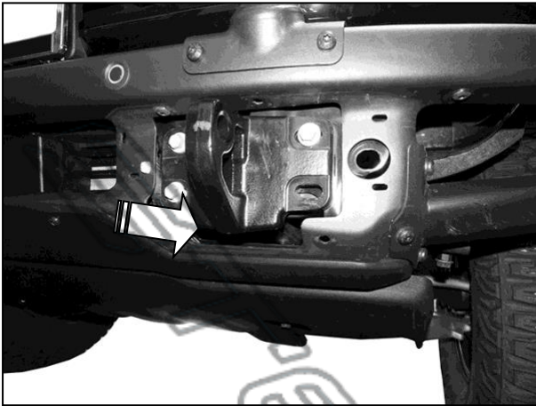
(Fig 7) Models with steel bumper, insert Upper Bracket between tow hook and opening in bumper (arrow). Attach end of Bracket to bottom of frame, between frame and splash guard bracket. Reinstall splash guard/skid plate and cover
