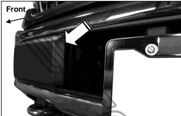
(Fig 1) From behind bumper, release metal clips attaching plastic bumper pad to the bumper
