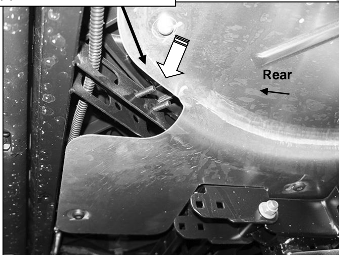
(Fig 6) Attach the passenger/right Support Bracket to the brace under the bed first, (arrow) then to the rear cross-member
