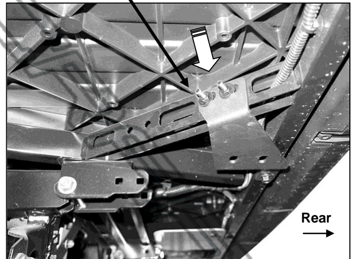
(Fig 2) Driver/left Support Bracket attached to brace on bottom of bed
