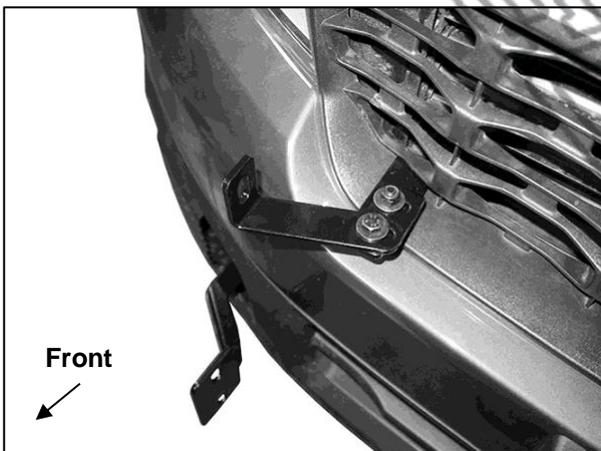
(Fig 20) Reattach the Top Outer Support Brackets (passenger/right side pictured)
