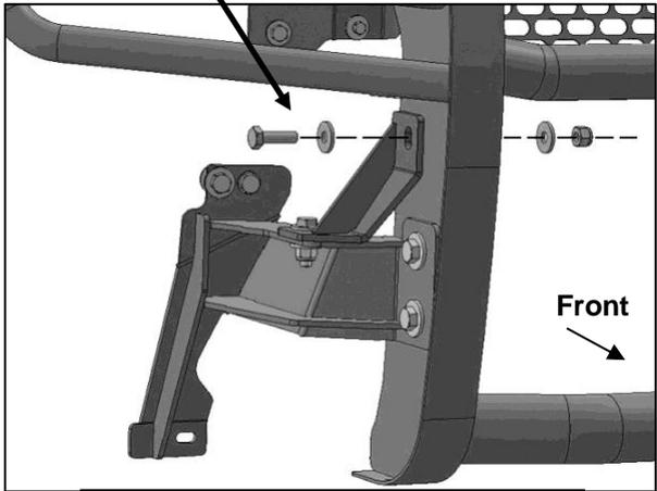
(Fig 23) Attach the passenger/right Lower Support Bracket to the outside of the Grille Guard
