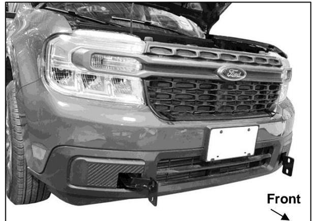
(Fig 19) Temporarily remove the Grille Guard from the Brackets.
