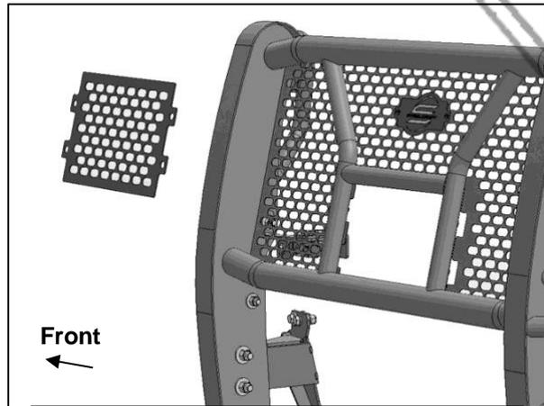
(Fig 24) Models with grille mounted camera, remove screen from Grille Guard
